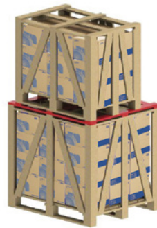
Figure 28 - Use of additional battens for stacking
