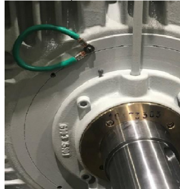
Figure 49 - Metal flexible braid
